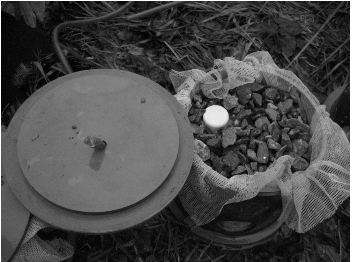
Figure 5.4. Picture of colonisation chamber containing coarse sediment with lid removed. Yellow data logger is shown inserted in the pot. The tube inserted in the lid is for extracting water samples while in situ. Boulling silk (63 \mu m mesh size) is visible on the end of the tube to prevent removal of taxa during water removal.
