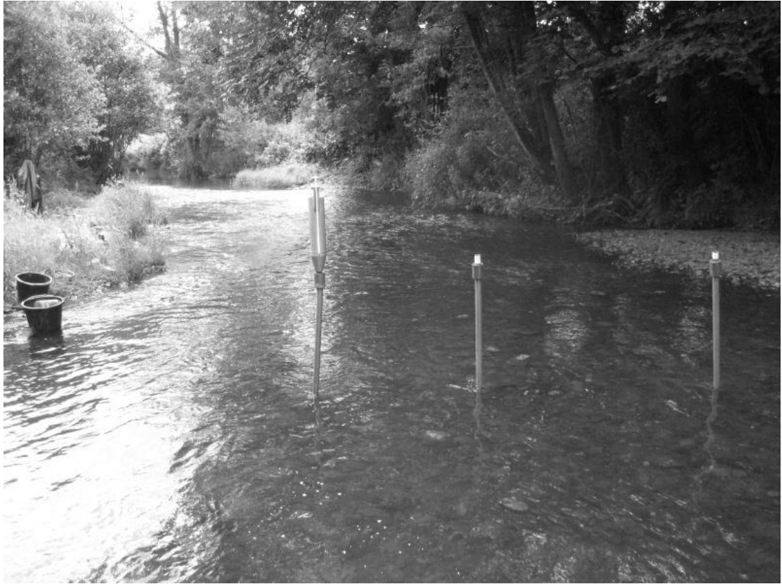
Figure 2:2. Example of piezometer distribution across a riffle head. Piezometers are set laterally across the riffle head and located at least 1 metre apart and more than 2 metres from the river bank. The BOU-ROUCHE pump is attached to the piezometer on the left. A similar distribution of minipiezometers was used to measure vertical hydraulic gradients. Water chemistry was taken using probes inserted directly into each piezometer.
